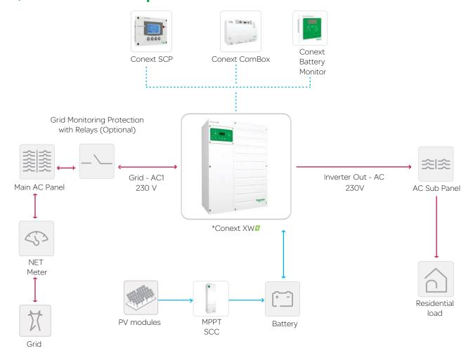
\*230 VAC solution with Conext XW+ 7048 (5.5 kW continuous backup, max 4.6 kVA sell) or Conext XW+ 8548 (6.8 kW continuous backup, max 6.2 kVA sell)
